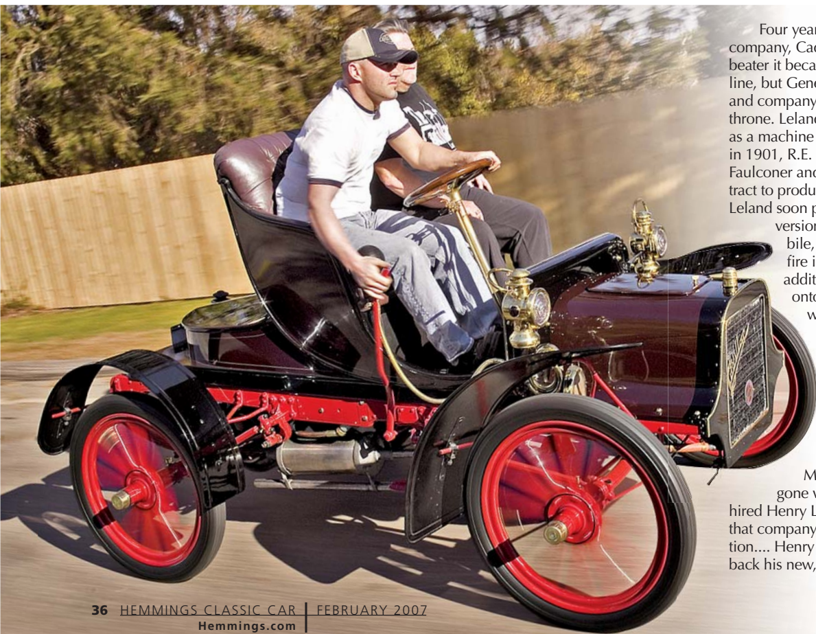
High and comfy, seats with ample room are a rarity in brass cars. Crank with anti-kickback safety starting device visible on the floor
