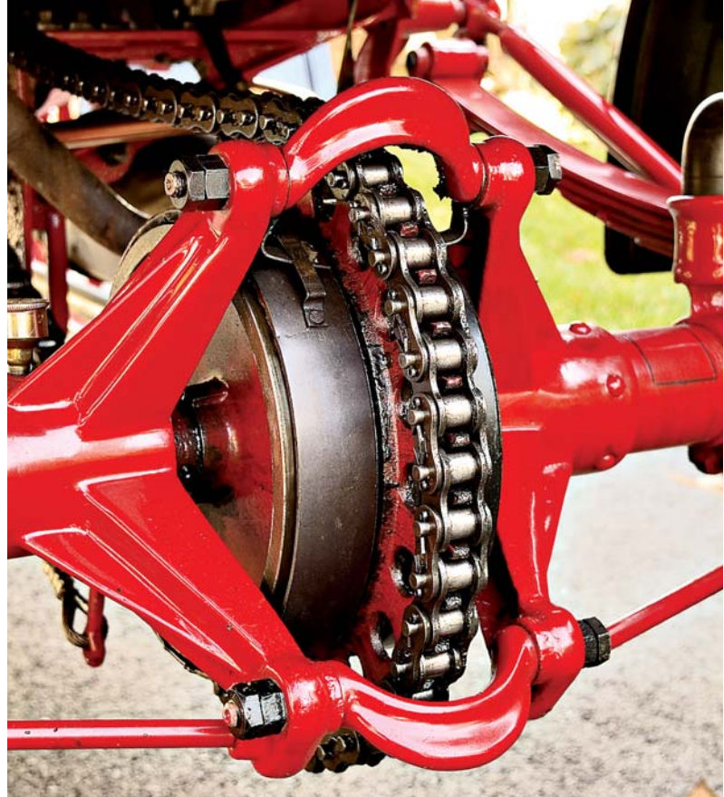
Ten-horsepower single drives two-speed planetary transmission to Brown-Lipe spur differential. Double-acting brakes inboard at rear
