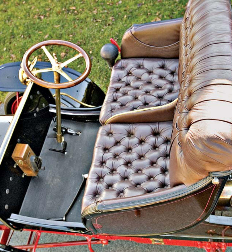
High and comfy, seats with ample room are a rarity in brass cars. Crank with anti-kickback safety starting device visible on the floor
