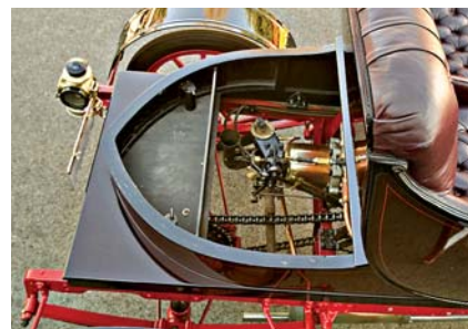
Iconic flat boattail rear decklid is held on from below with twin clips
