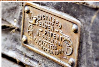
Badge for Selden patent on internal combustion engine, beneath seats
